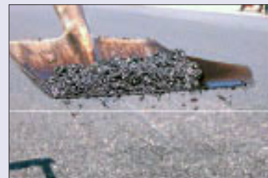
Hot mix asphalt and aggregate with FORTA fibers hanging from shovel
